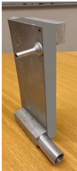
Figure 2-57: Prototype internal heat exchanger, design based on the experiences from the one shown in Figure 2-54.
