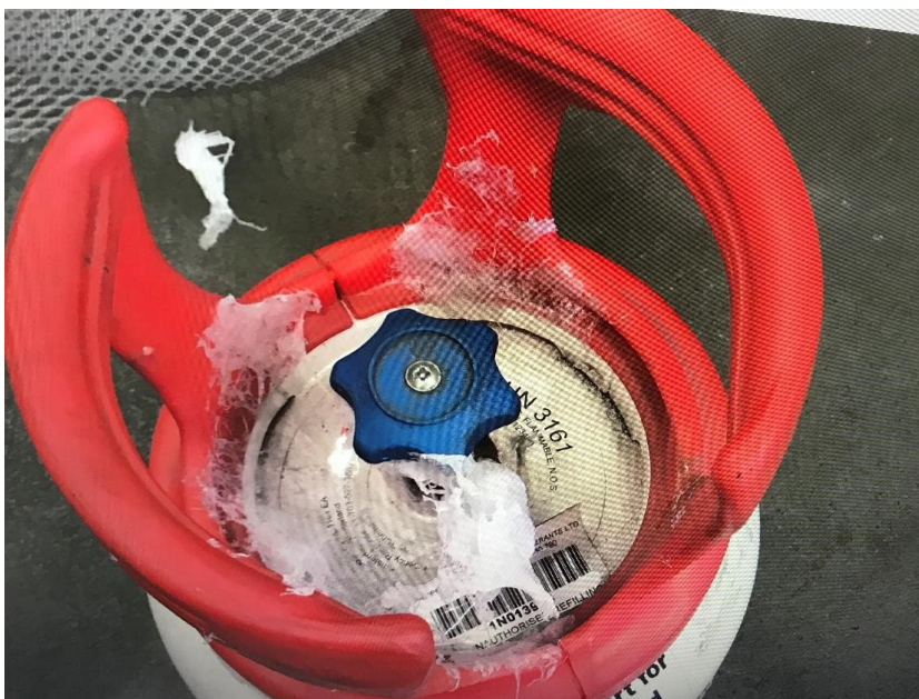
Figure 2-51: Bottle of R513A giving off a white foam when the valve is opened.
