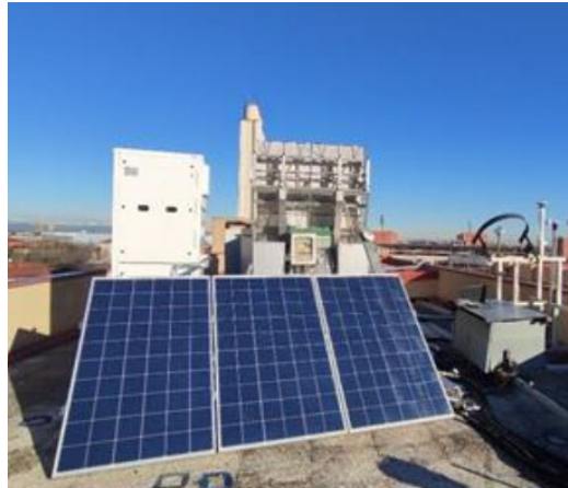
Figure 3-14 - Solar assisted heat pump prototype working with CO 2 installed at the Solar Energy Conversion Laboratory (Department of Industrial Engineering, University of Padova).
