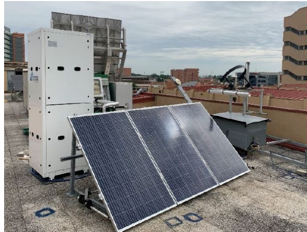
Figure 3-6: Solar-assisted heat pump prototype was installed at the Solar Energy Conversion Laboratory (Department of Industrial Engineering, University of Padova).
