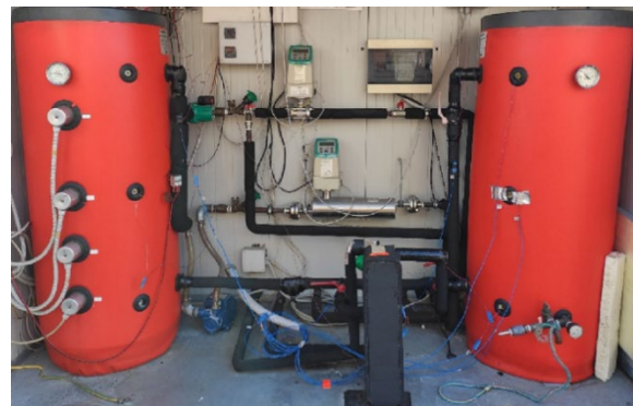
b. Picture of water tanks, brazed plate heat exchanger and flow meters installed in the water loop.
