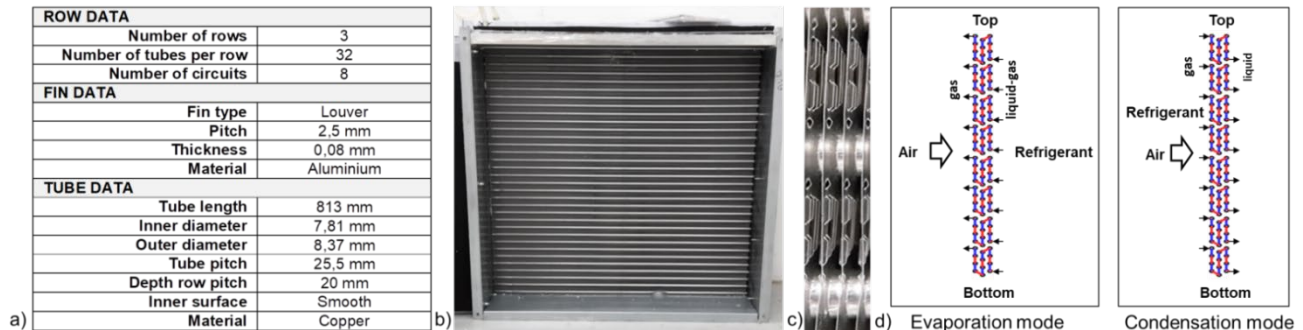
Figure 4-26: Main characteristics of the tested finned tube heat exchanger: a) Geometry characteristics; b) Overview photography; c) Fins close-up; d) Flow patterns
