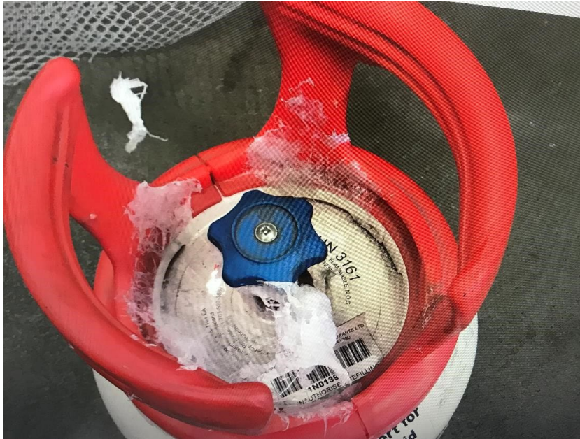
Figure 2-51: Bottle of R513A giving off a white foam when the valve is opened.
