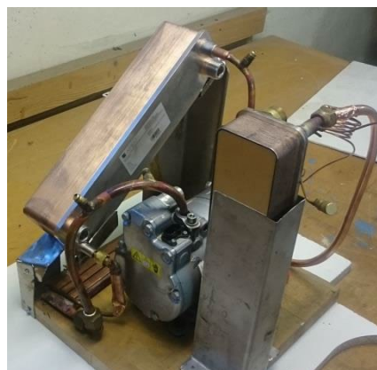
Figure 2-3: Low charge propane heat pump, 2 - 10 kW capacity. Basic components during construction.
