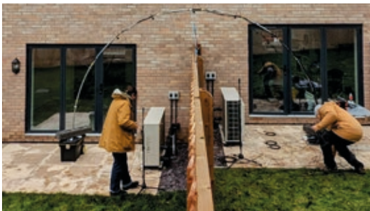
Figure 2: A pair of ASHPs, located in the gardens of two new build houses in Nottingham, UK, were measured using a 180° microphone arc. 9 microphones were mounted on the arc, in order to observe interactive effects from the ASHPs caused by their close proximity. [Source: USAL, Heat Pump Association]
