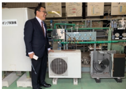
First prototype of the Eco-Cute heat pump for domestic hot water heating, using CO 2 as refrigerant.
