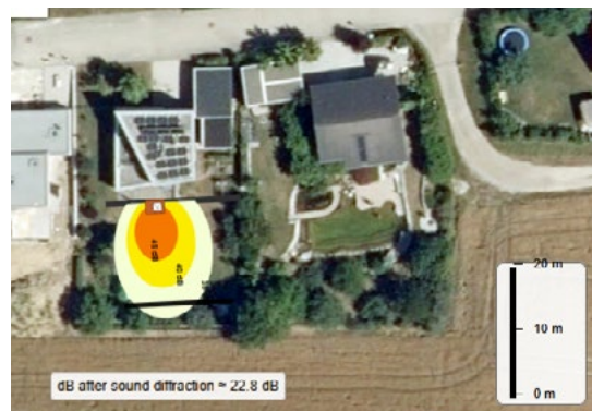
Figure 2: Result from enhanced web-based tool to enable sound propagation assessments for residential heat pump planning.
