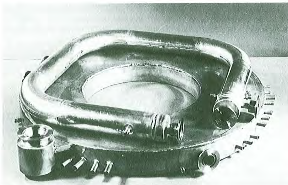
Figure 4. Bubble absorber with internal heat exchanger
