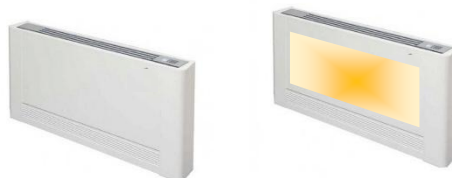
Figure 9 – Image for pure illustrative purpose, non-exhaustive, of very widely diffused solutions for forced air convection (from left to right: ultrathin floor standing application with casing and with additional integrated radiant heating function) for heating and cooling application using cold or hot water (e.g. 7-12°C in summer and 45-40°C in winter) as thermal vector to provide heating in winter season and cooling in summer season. The radiant heating function helps improve the heating comfort compared to traditional Fan Coils.
