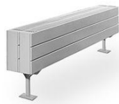
Figure 5 – Image for pure illustrative purpose non-exhaustive, of a typical convactor normally used for large spaces: very widely diffused for heating only application using water as thermal vector generating localized convection flows of air indoor, normally without filtering function.
