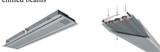
Figure 10 – Image for pure illustrative purpose, non-exhaustive, of very widely diffused solutions (especially in northern Europe) for chilled beams (from left to right: active type with also air renewal and purification integrated supply from central AHU / HRU and passive type) for heating (and, in many cases, also cooling) application using water at moderate temperatures (e.g. 18-23°C / 35-30°C) as thermal vector to provide heating function in winter season and cooling function in summer season.
