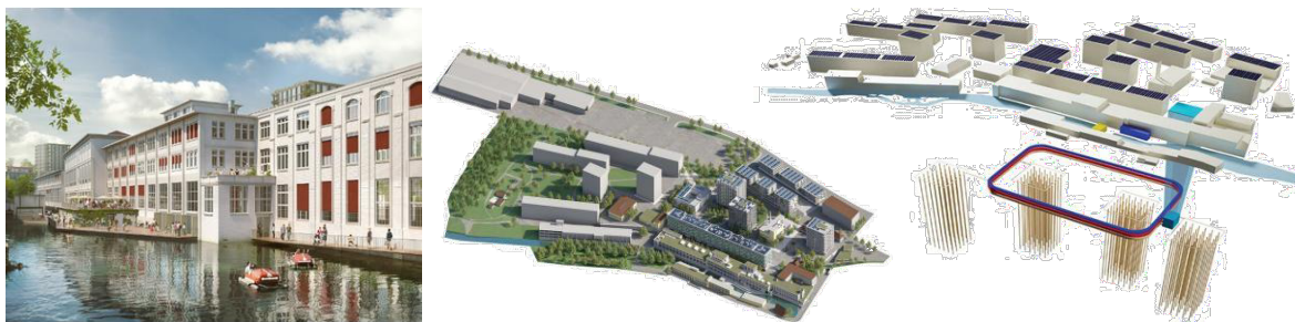
Figure 8. View of the Papiéri District from the river Lorze (left), development state (middle) and energy concept with borehole fields and river water heat source for the centralized HP
