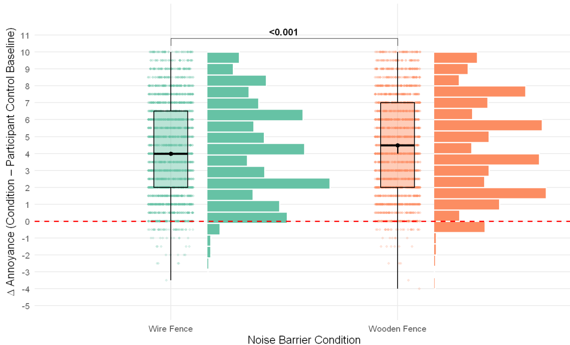
Figure 3. Baseline-corrected annoyance ratings for the wire fence and wooden fence conditions. The red dashed line at zero represents the ambient-only baseline; values above zero indicate increased annoyance due to the ASHP. The bracket indicates a statistically significant difference between conditions ( p < 0.001 , Wilcoxon signed-rank test).
