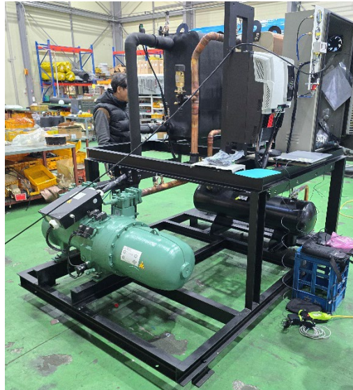
Figure 7. The constructed screw chiller
