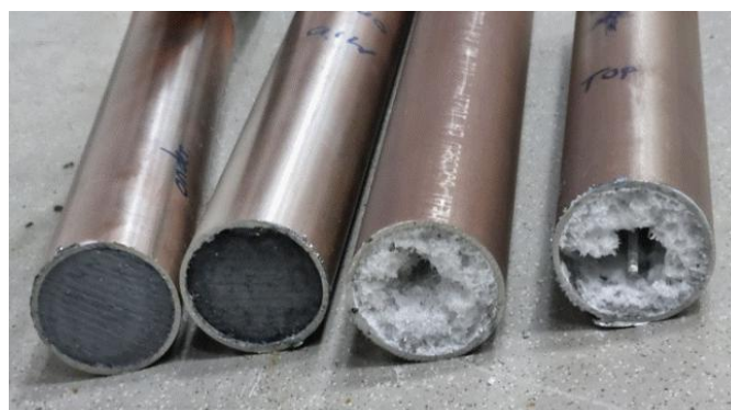
Figure 5. Post test analysis of LHTES tubes with adipic acid/graphite mixture, showing two sections of the tube, in the middle (left tubes) and at the top (right tubes).
