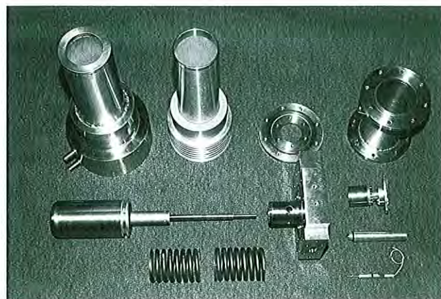
Ready to assemble: the Stirling engine is made from these simple components.
