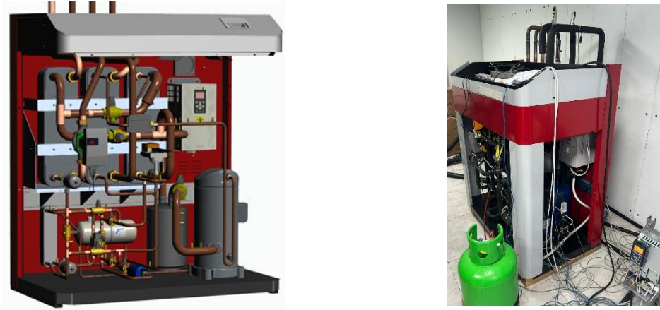
Figure 4: 3D CAD picture of the HTHP (left) and photo of the HTHP during testing (right)
