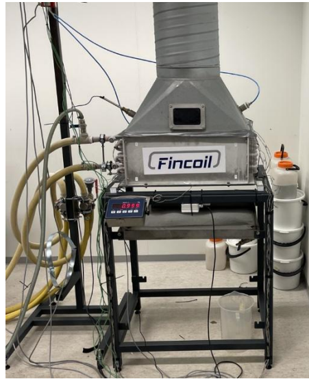
Figure 1 The laboratory-scale test setup with coil size of 595 mm x 420 mm x 182 mm [9]
