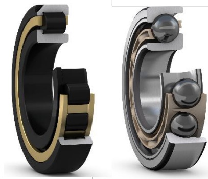
Figure 2. Typical bearings used in heat pump applications — Left: cylindrical roller bearing with tribological black oxide coating; Right: hybrid angular contact ball bearing with ceramic rolling elements and stainless-steel rings [8]
