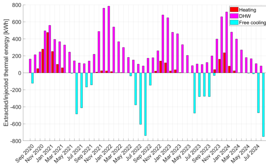
Figure 3. Monthly thermal energy extracted from or injected into the ground from September 2020 to August 2024.
