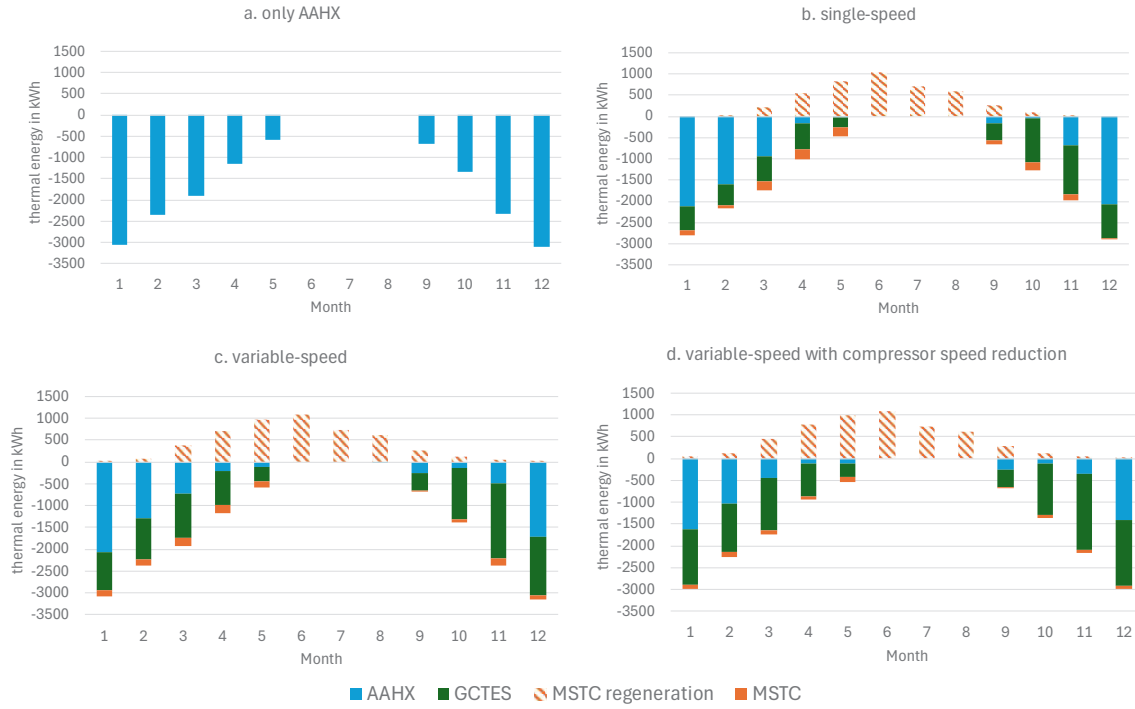
Figure 10. Thermal energy for all heat sources and monthly average COP.
