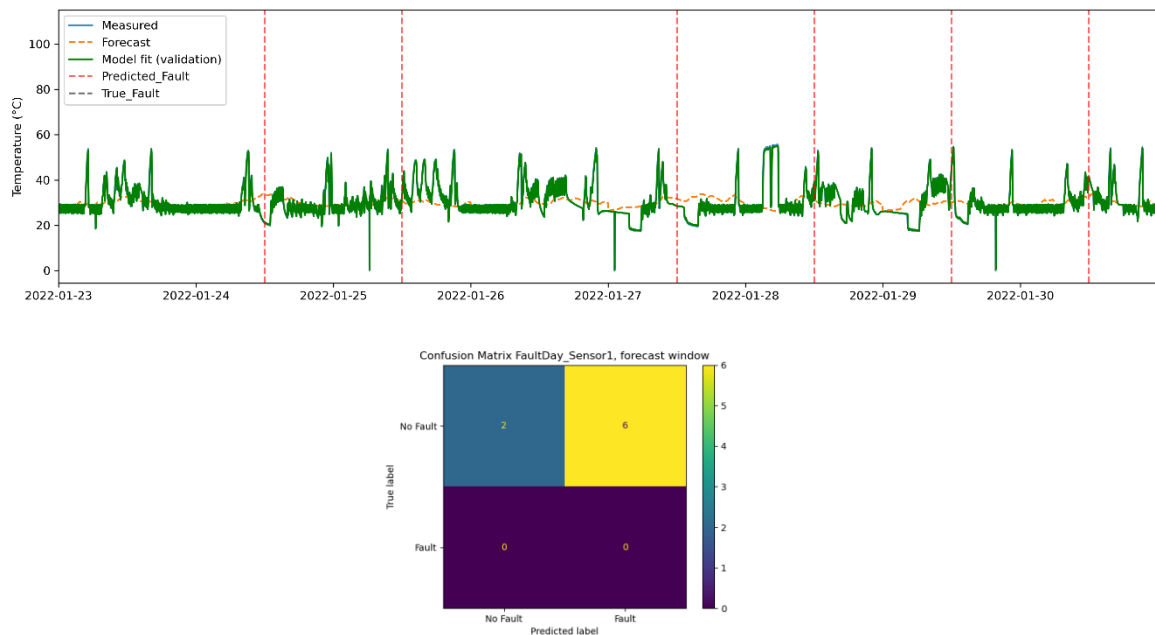
Figure 3. Results for 8-days testing of the ML-Pipeline on winter days in January for HP-System 2
