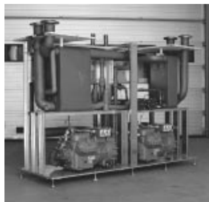
▼ Figure 2: Chiller pack.
