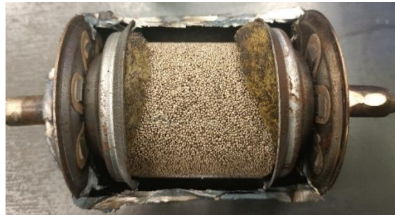
Figure 3. A dissected liquid line filter (length: approx. 10 cm).
