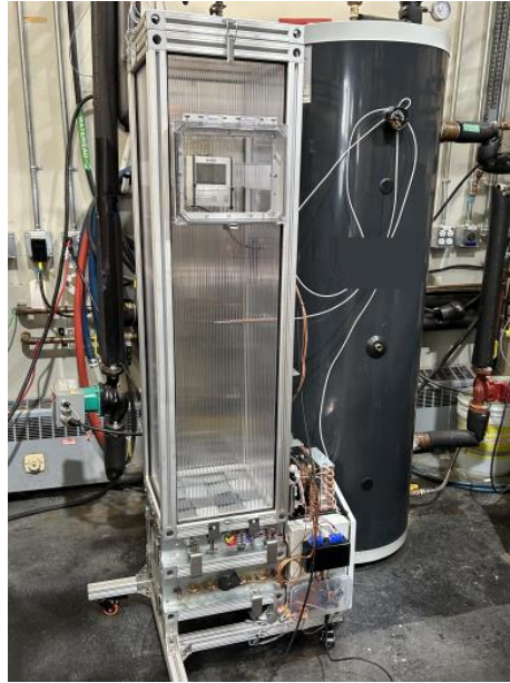
Figure 2. Thermostat environment emulator (TEE) installed in the main laboratory area
