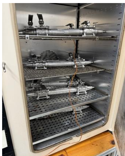
Figure 1. Metal gas reactors with refrigerant samples during thermal stability tests in the lab oven (21 days).
