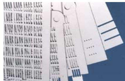
This photo shows a compact heat transfer surface studied in Annex 33
