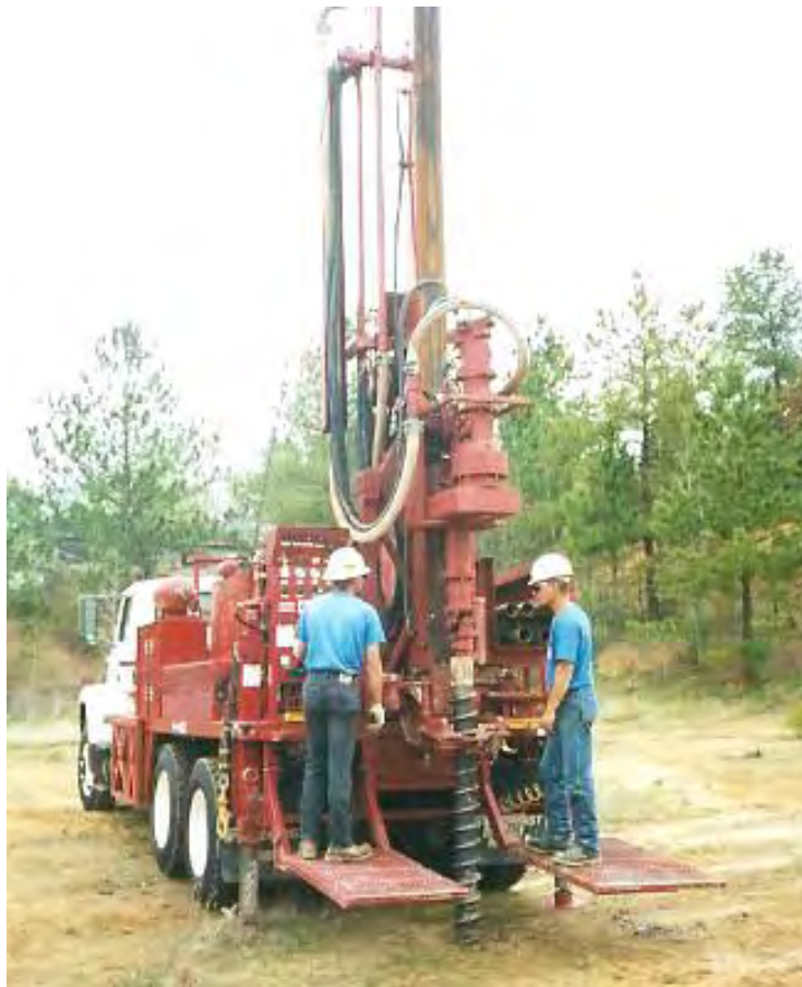
Fig. 5.34: Rotary Drilling
