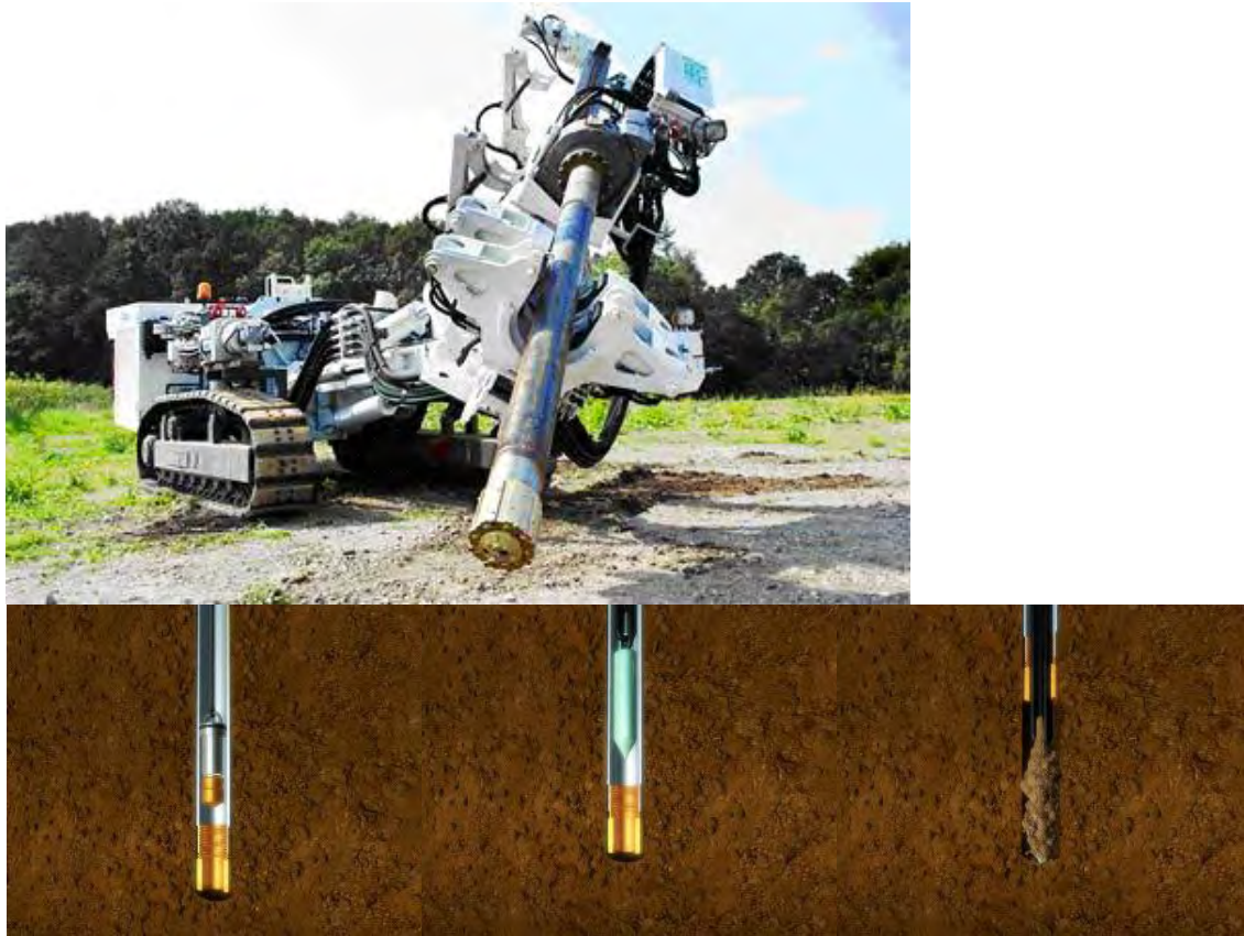
Fig 5.35: GeoJetting Rig and Method
