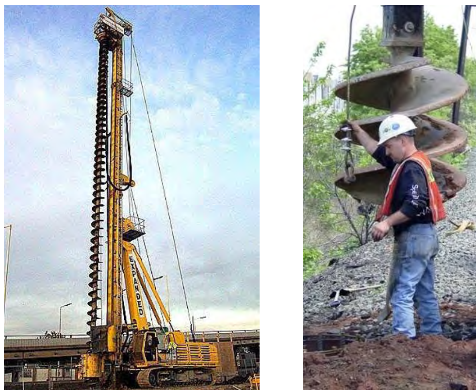
Fig. 5.35: Auger Drilling Equipment
