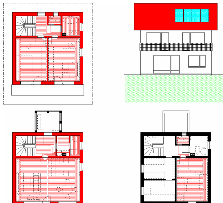
Fig. 5.12: Single-Family House with a Floor Heating System
