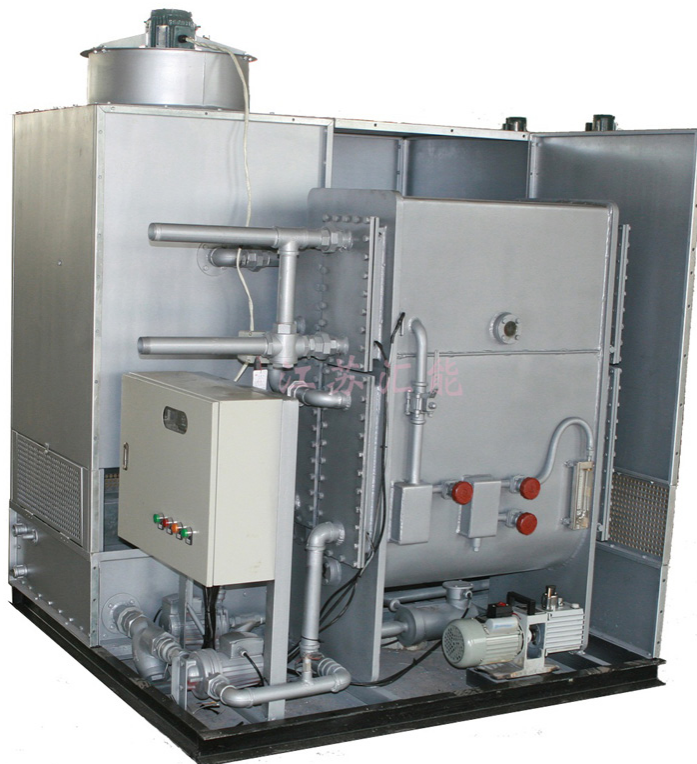
Figure 1: Integrated absorption system with 23 kW water/lithium bromide absorption chiller, wet cooling tower and pumps. (Source: Jiangsu Huineng)
