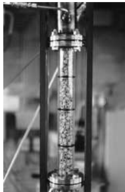
▲ Figure 2: Close-up of a mass transfer unit, height = 50 cm.
