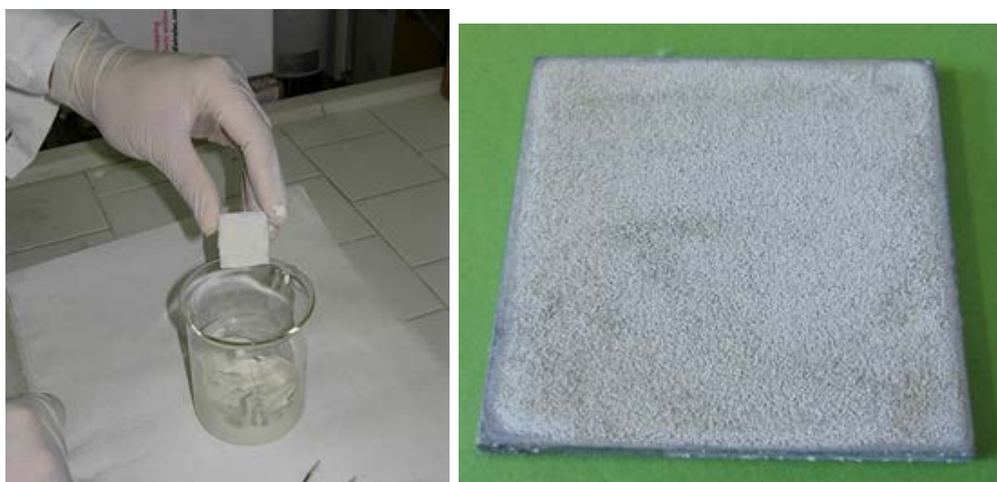
Fig. 3-3: Preparation of the coated samples: dip coating phase and consolidate layer after calcination.
