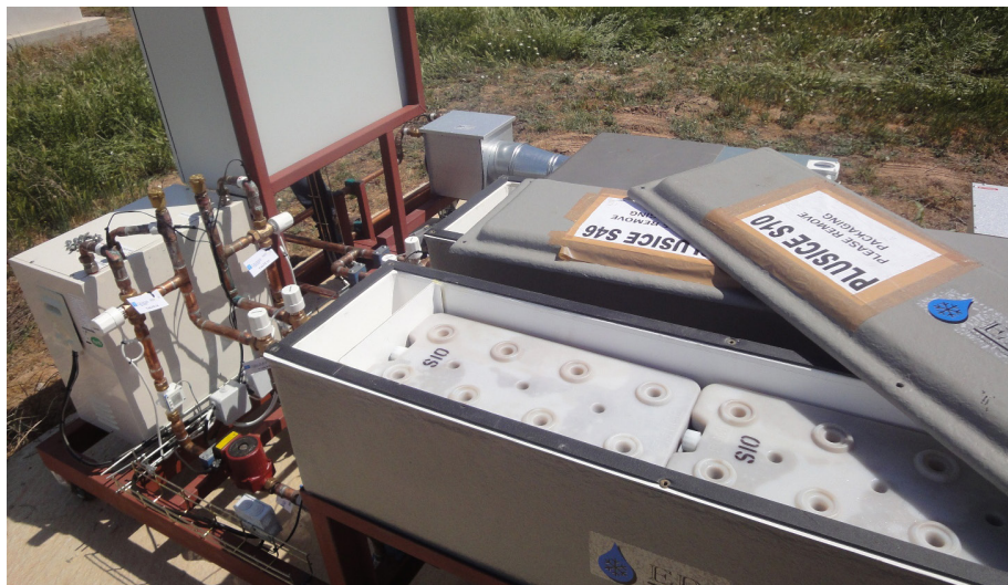
Figure 4. PCM thermal energy storage tanks
