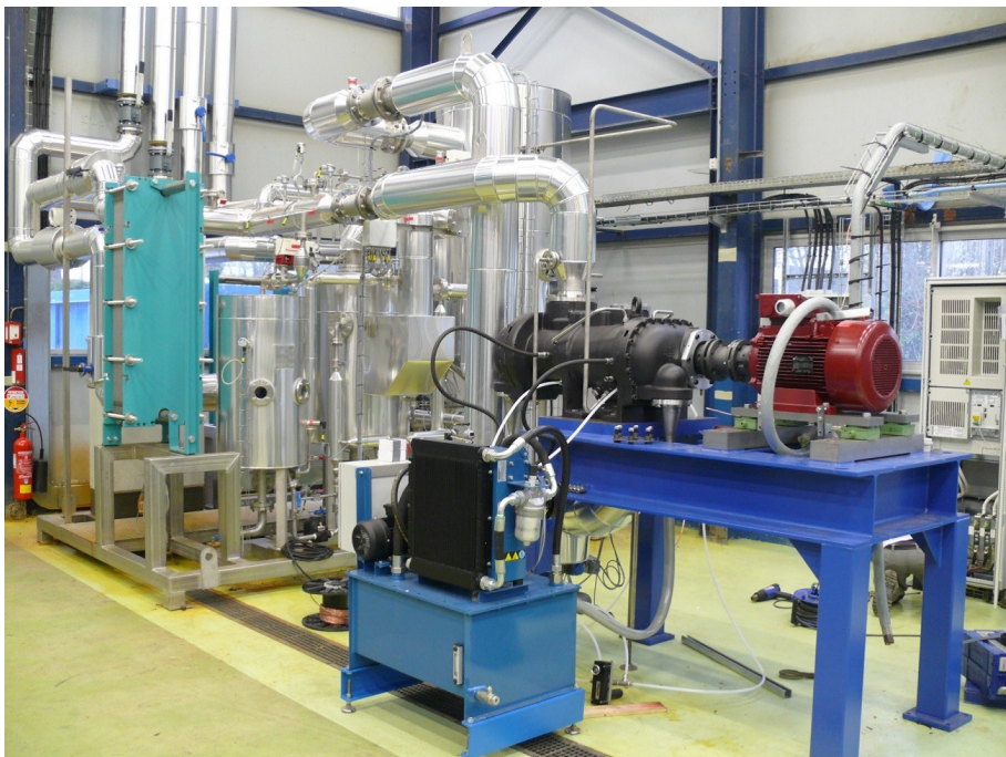
R&D: VHT heat Pump, up to 140 °C, with water as working fluid (Source: EDF R&D)
