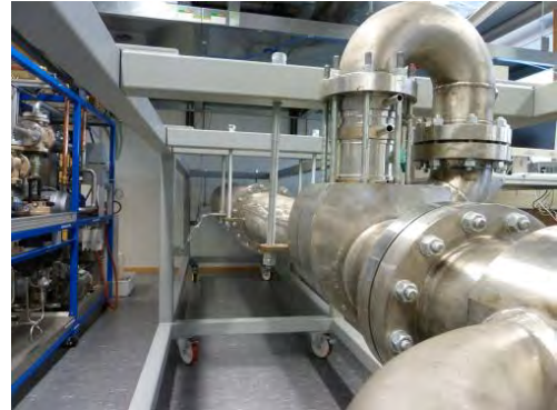
Figure 10-9: Thermo acoustic heat transformer at ECN
