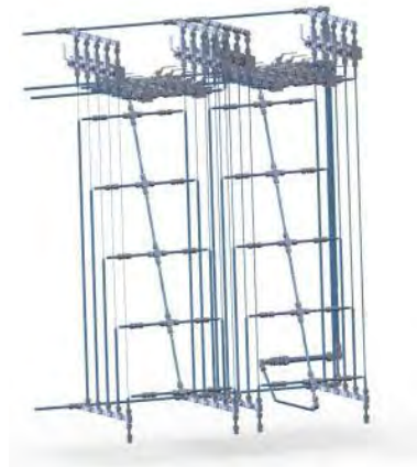
Figure 10-16: Mini channel heat exchanger
