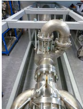
Figure 10-9: Thermo acoustic heat transformer at ECN
