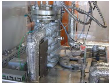
Figure 10-10: Thermochemical heat pump transformer
