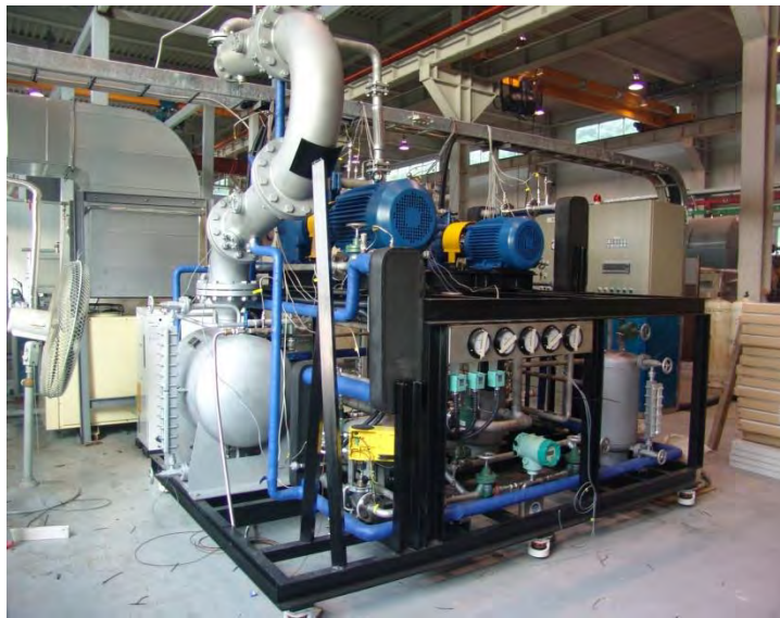
Figure 9-2: Prototype of a compression/absorption heat pump system
