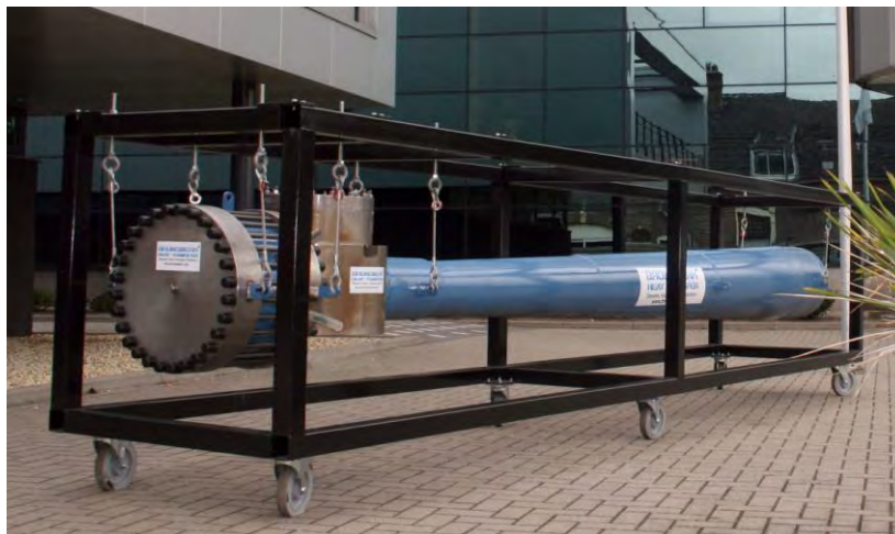
Figure 10-14: Electrically driven thermoacoustic system
