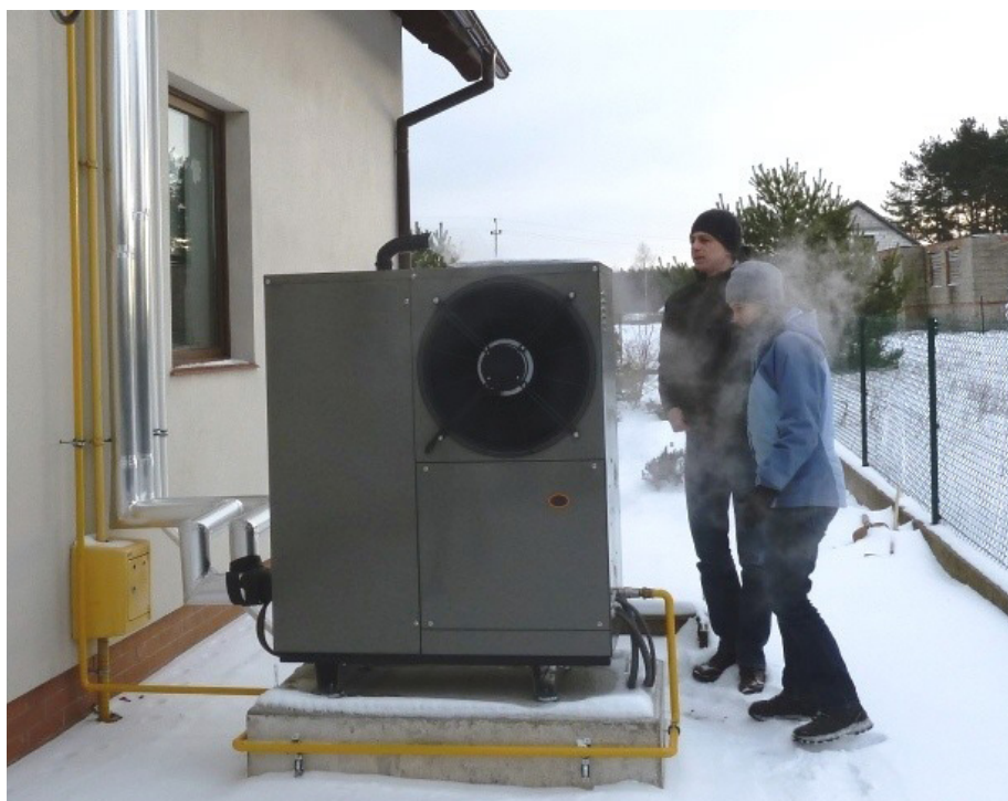
Annex 43: Field test of a new prototype of an absorption heat pump.
