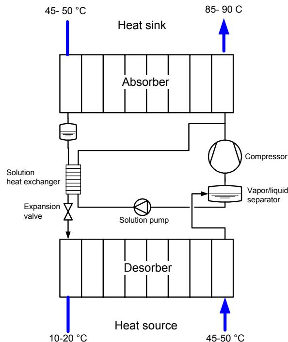
Figure 1: Hybrid heat pump sketch
