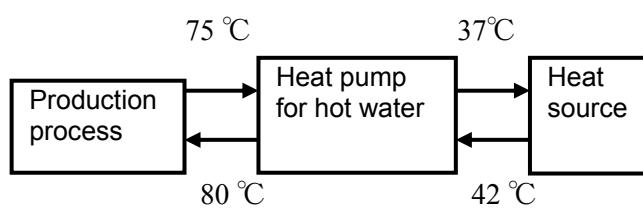
Figure 2: Facilities the heat pump
