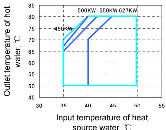
**Figure 4: Performance curve of coefficient of performance**
