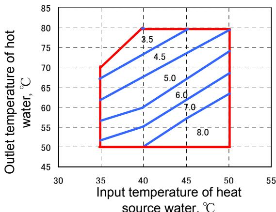
**Figure 3: Performance curve of heat output**
