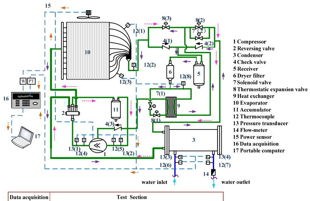
**Figure 1: Schematic of the field test system**
