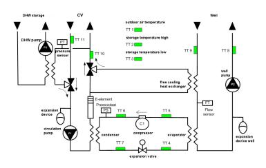
Many self contained heat pumps will already have temperature and pressure measuring points, an energy consumption meter and some form of data logging. This data will typically be used for maintenance and servicing of the heat pump itself. But the performance of the system is also strongly dependent on changes in the source temperature, the properties of the building or apartment and user behaviour.
