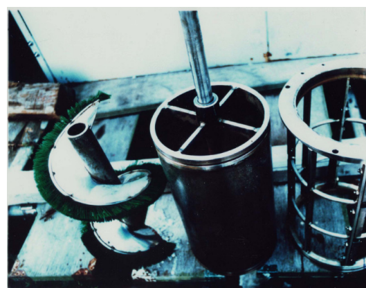
Figure 12 Inside of auto strainer
