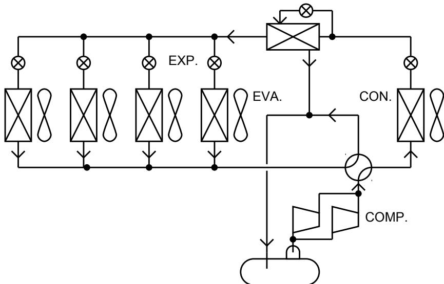
Figure 1: Schematic flow of VRF system
