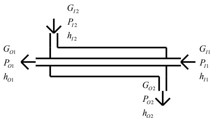
**Figure 4: Sub Cool Heat Exchanger**
