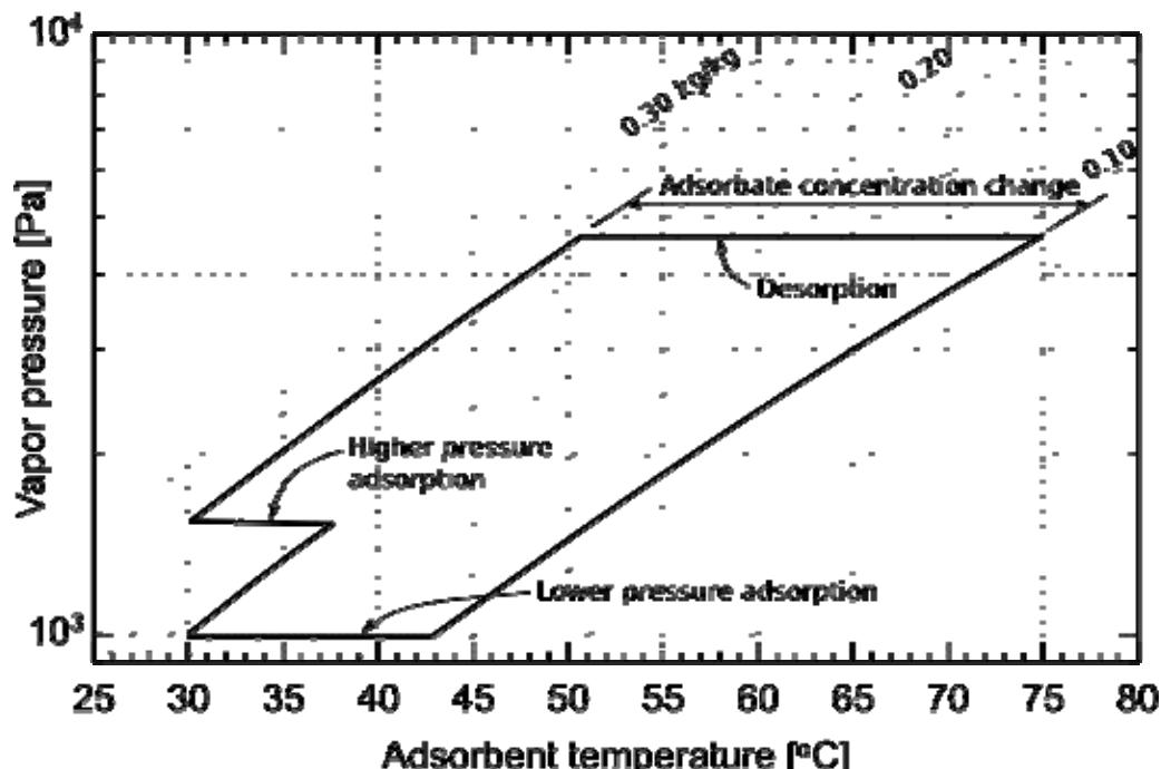
Figure 3: The adsorption cycle of the DEAC.
