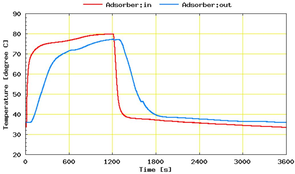
**Figure 5: The inlet and outlet temperatures of the adsorber.**
