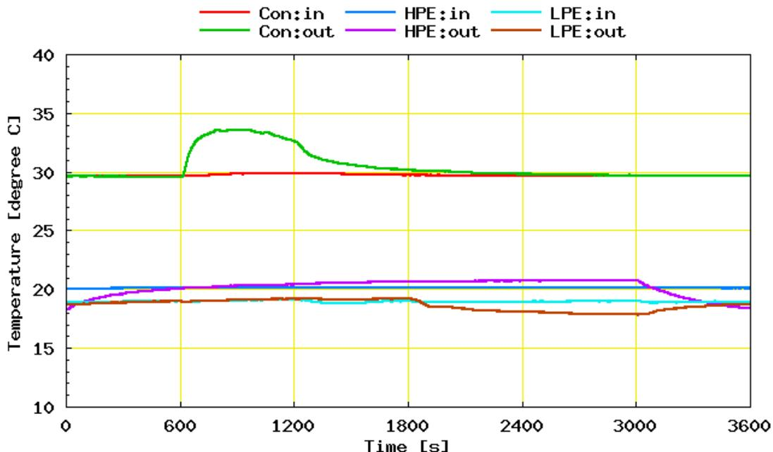
**Figure 6: The inlet and outlet temperatures of the condenser and the evaporators.**
