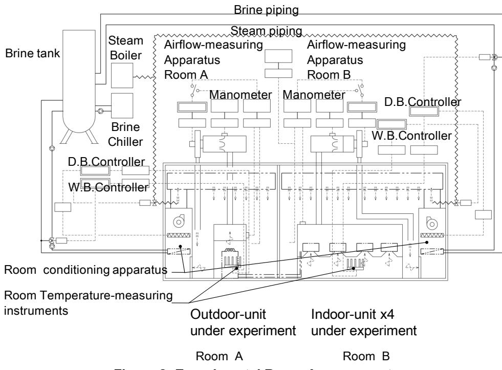
**Figure 2: Experimental Room Arrangement**
