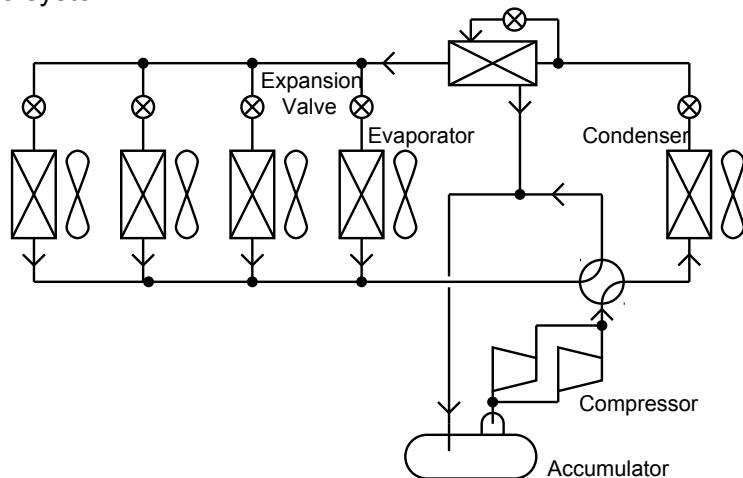
**Figure 1: Refrigerant circuit arrangement (Cooling)****Table 2: Published specification of the system (60Hz) under rating capacity condition**
