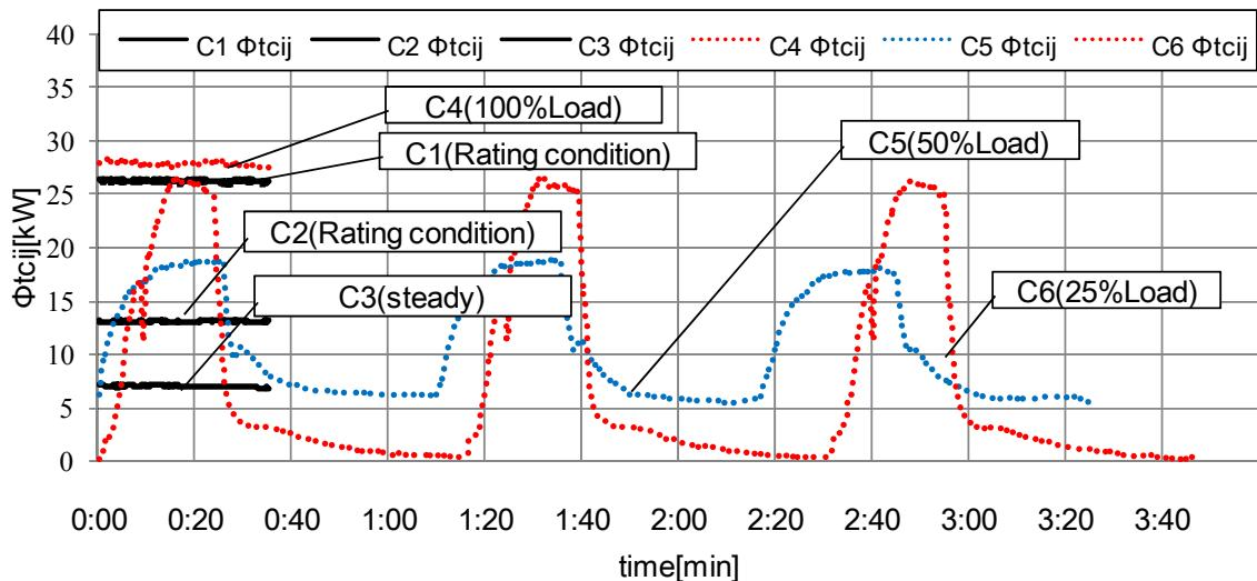
**Figure 5: Total heat exchange on indoor units (cooling)**
