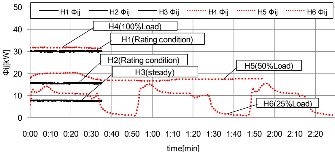
**Figure 6: Total heat exchange on indoor units (heating)**
