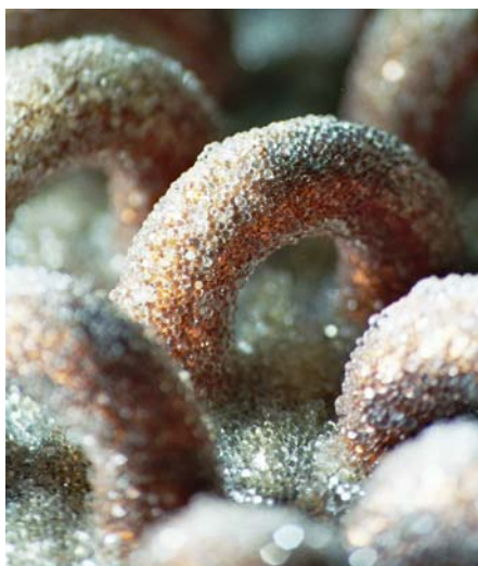
Figure 2: Photo of a silica gel coated tube and fin adsorber heat exchanger
