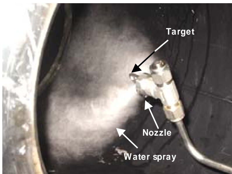
Figure 4: Plume characteristics at operating pressure of 7 MPa
