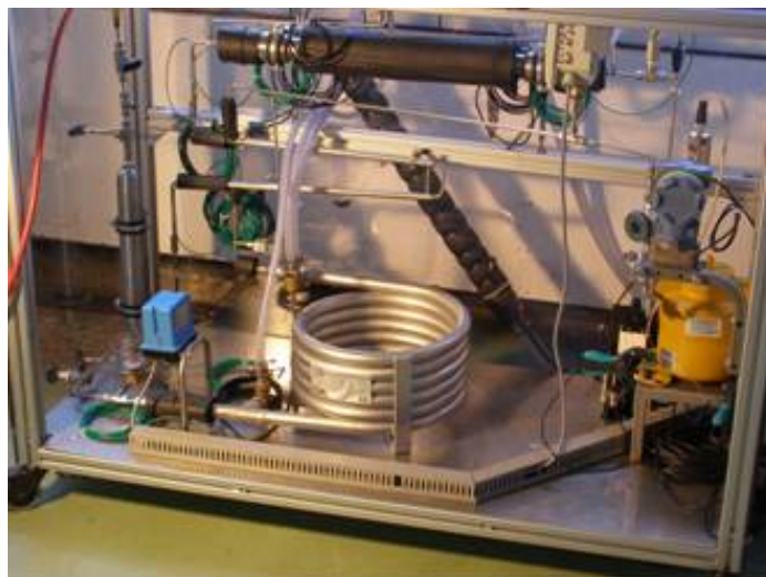
Figure 2: Overview of the CO 2 heat pump prototype.
