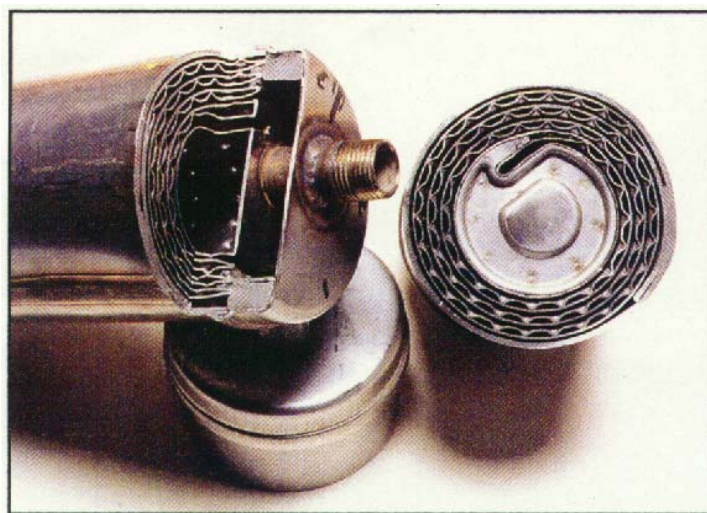
Figure 3: Spiral plate heat exchangers (Spirec).
