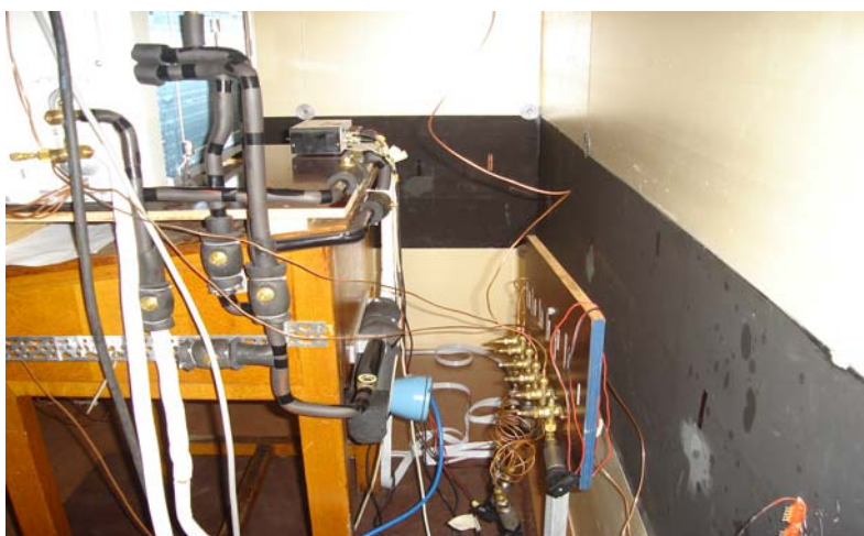
Figure 5: Flow-meter integrated in the refrigerant circuit
