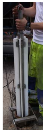
Figure 4: Flow logging probe insertion into the borehole
