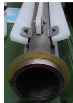
Figure 5: Flow logging probe
