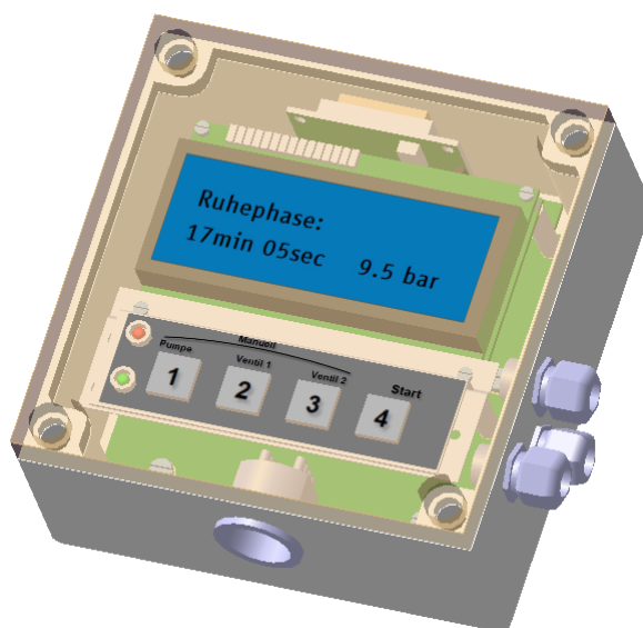
Figure 5: Device to perform automatically the borehole heat exchanger contraction procedure for tube tightness testing.
