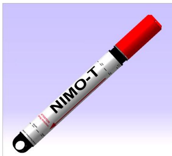
Figure 1: NIMO-T: Wireless tool for continuous temperature measurements in borehole heat exchangers. See Table 1 for technical details.
