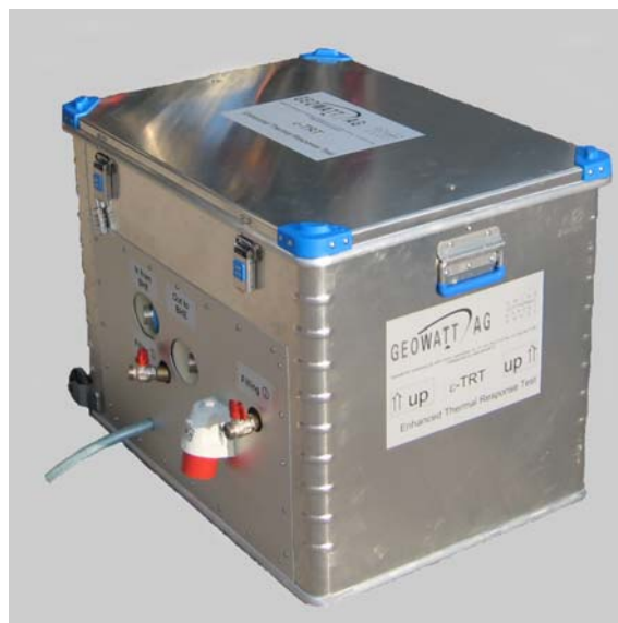
Figure 4: Geowatt eTRT device. The power is continuously adjustable from 0 to 10 kW. Power and circulation can be regulated independently. The accuracy of electrical and hydraulic power measurement is 1% and 1.5%, respectively.
