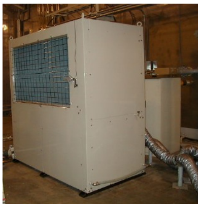
Figure 2: the Developed Heat Pump Tested in the Climatic Environmental Testing Room
