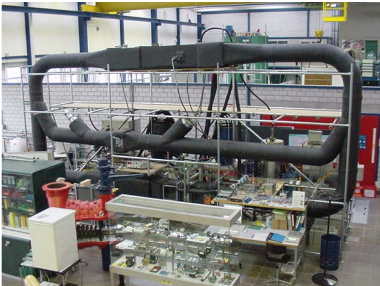
Figure 2: Pilot plant test facility for air cooled evaporators [Berlinger et al., Sahinagic et al.
