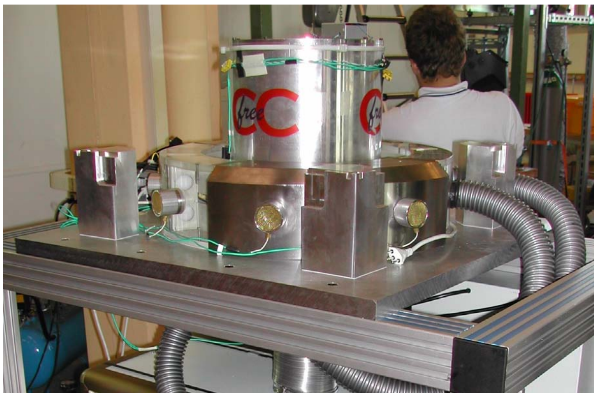
Figure 4: Prototype of a refrigeration machine with magnetic thermo-cycle [Sari et al. 2007]
