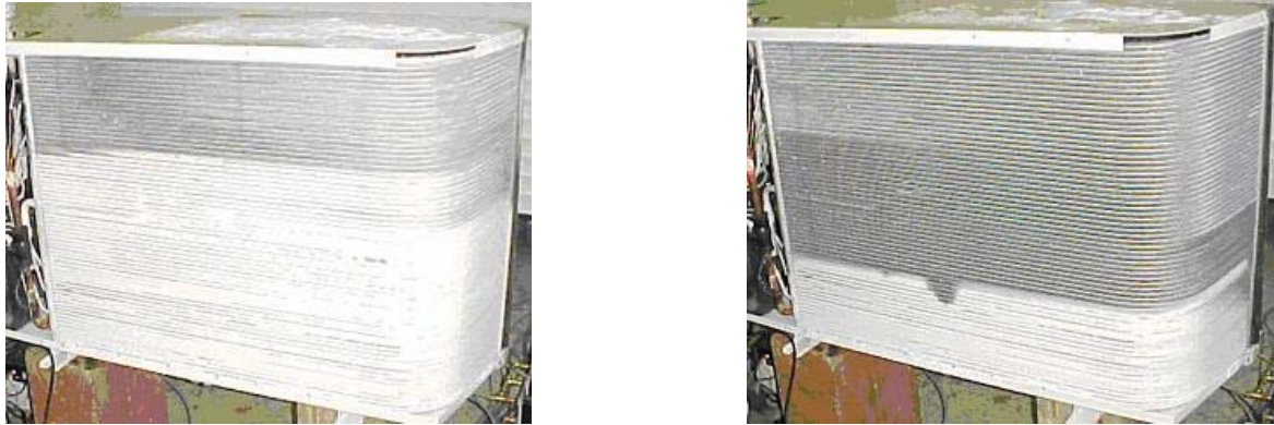
Fig. 9. MCHEx defrosting behavior (after one minute at the left, and three minutes at the right).
