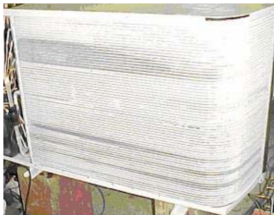
Fig. 8. MCHEX aspect after 30 minutes of frosting.
